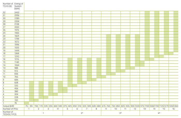
\* From eight TS HV 80 per TESVOLT PCS, an external DC combiner is required. This is not part of TESVOLT's scope of delivery and is to be configured on a project-specific basis.
